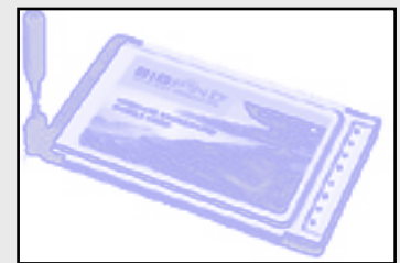
Telstra's 1x-EVDO PC Card. Plug one into a laptop PC and you're connected at up to 512 kbps, where full speed services are available - and around 100 kbps where they're not.
