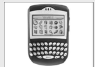
The BlackBerry 7250 Handheld Unit. Telephone, e-mail and wireless modem. Internet access to your laptop at up to 600kbps on Telstra's 1xEVDO network (100kbps on some regional CDMA networks).
